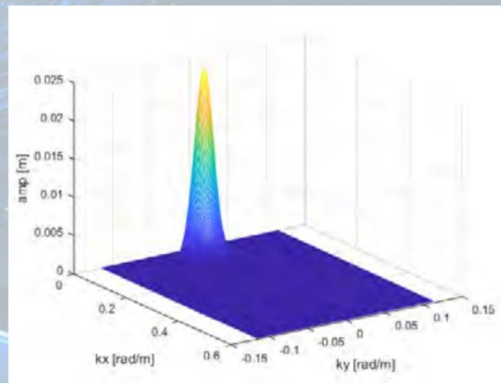
Figure: Input JONSWAP wavenumber spectrum
