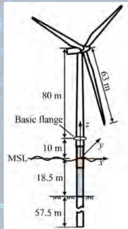
Figure: Monopile foundation (Mo et al., 2017) 3 / 30
